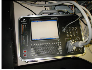
Recording traffic using a SCSI bus analyzer.
