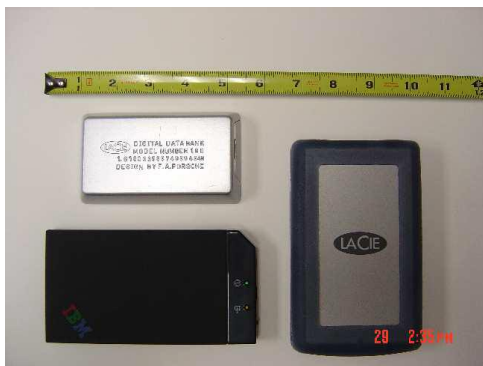
Figure 2: A sample of USB 2.0 portable disks used as SoulPads . Clockwise from upper left: LaCie 40GB DataBank, LaCie 60GB PocketDrive, and IBM 40GB Portable Hard Drive.
