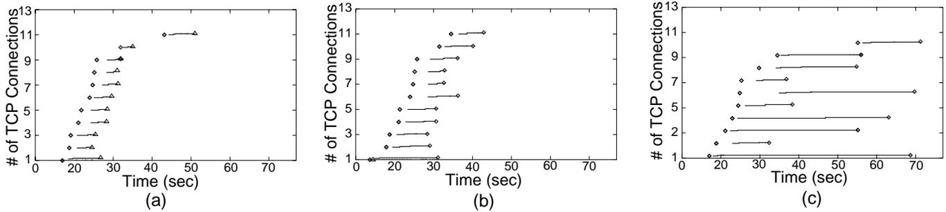
**Figure 11: HTTP time line sequence for each wireless interface while downloading CNN top-level page. a) Opt1, b) Opt2, c) Opt3. Each small rise in the lines represent a separate GET request made using that specific TCP connection.**
