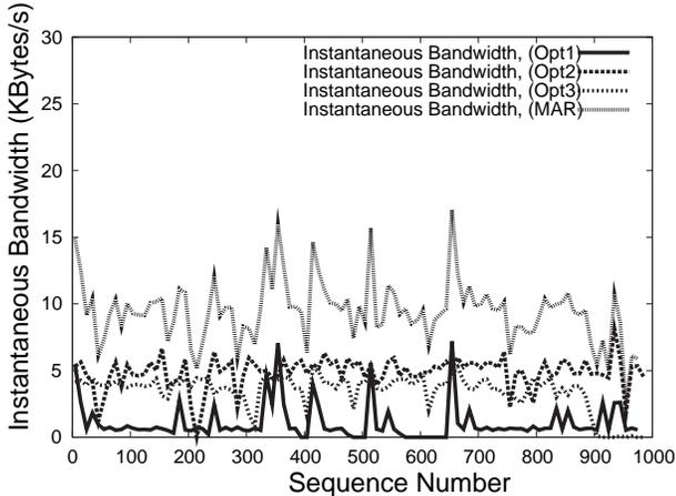
Figure 9: MAR UDP Performance. Mobile environment. Throughput for each interface stand alone, and for MAR
