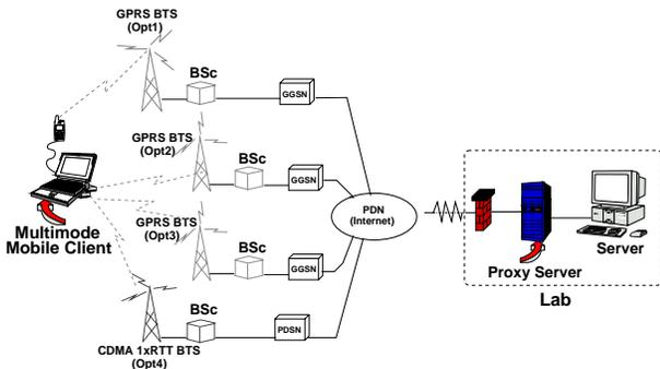
Figure 2: Experimental Set-up for Diversity Experiments with TCP.
