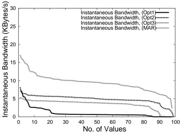
Figure 10: MAR UDP Performance. Mobile environment. Aggregated sorted throughput.
