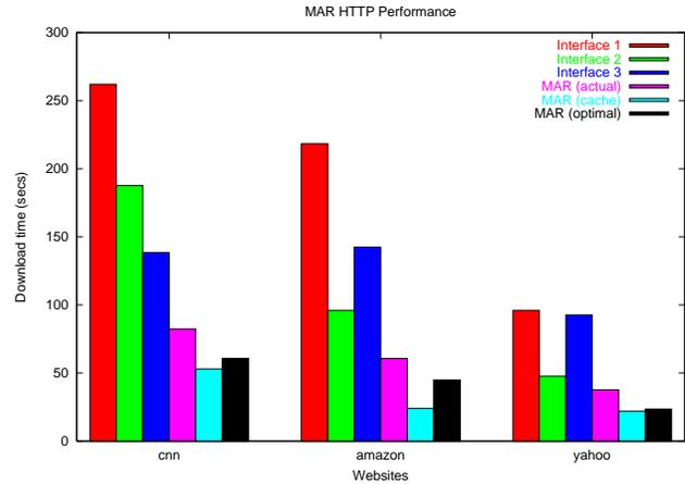
**Figure 12: MAR HTTP Performance. Latency for different Web sites where the first three columns in each set represents the performance of each operator stand alone, next one is MAR (current implementation), next one is MAR with caching, and the last one is MAR (ideal).**
