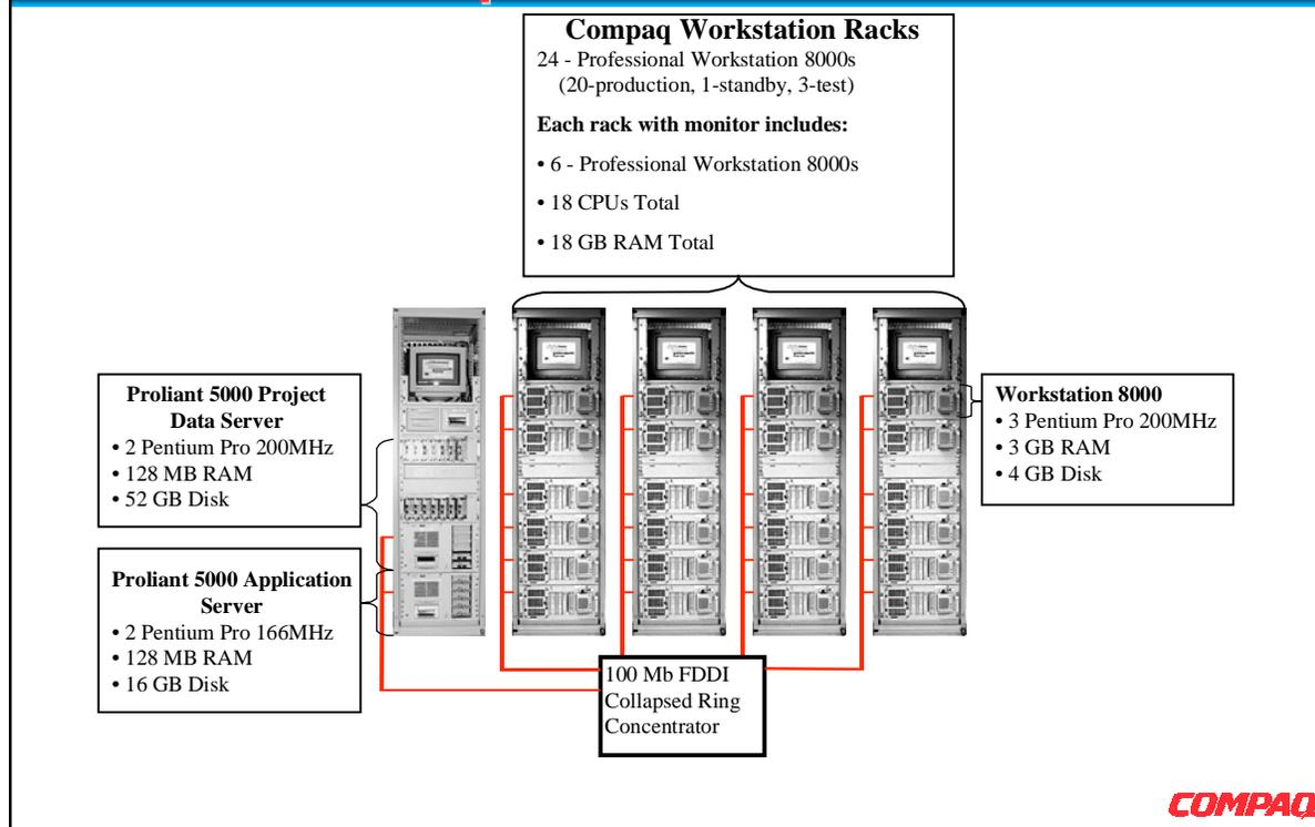
**Figure 3. Compaq's Windows NT Compute Farm Configuration**
