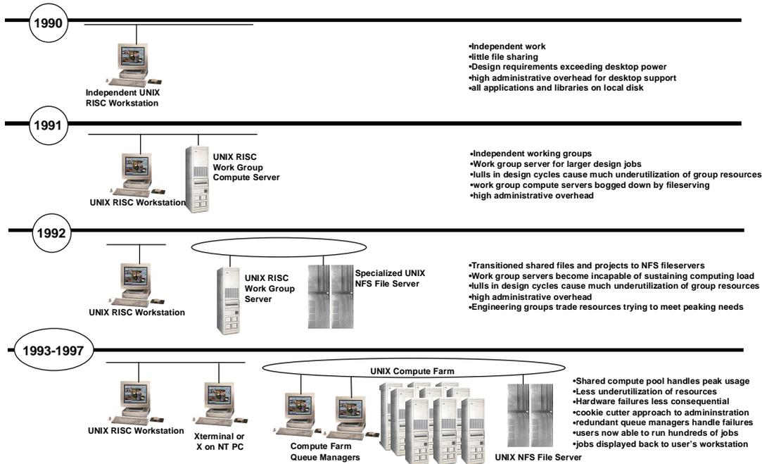
**Figure 1. Evolution of Compaq's UNIX-based Compute Farm**
