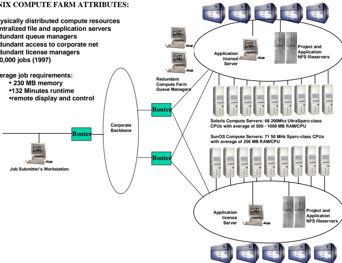
**Figure 2 Compaq's UNIX-based Compute Farm**
