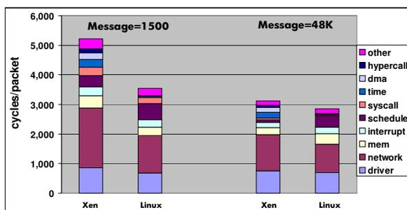
Figure 3: Kernel CPU cost for direct I/O
