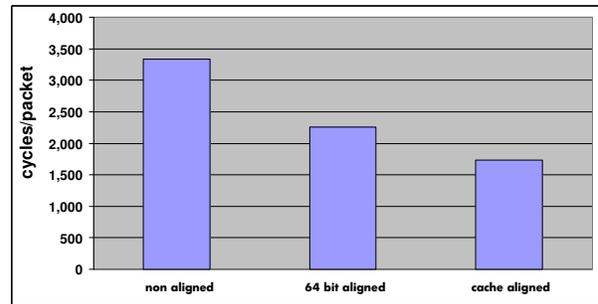
Figure 4: Alignment effect on data copy cost
