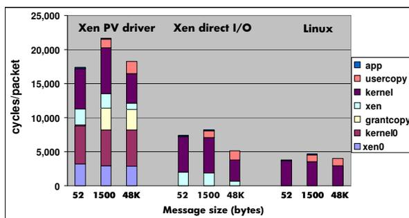
Figure 2: CPU usage to receive UDP packets
