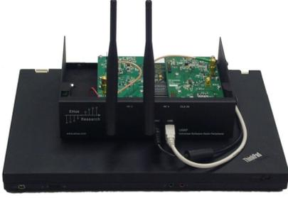
Figure 11: Experimental hardware setup of the UDSSS implementation, consisting of a Universal Software Radio Peripheral (USRPs) and a Lenovo T61 ThinkPad.
