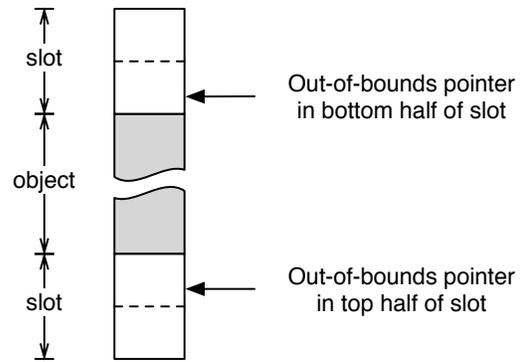
Figure 4: We can tell whether a pointer that is out-of-bounds by less than  $slot\_size/2$  is below or above an allocation. This lets us correctly adjust it to get a pointer to the object by respectively adding or subtracting  $slot\_size$ .
