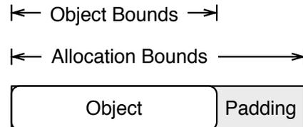
Figure 1: Allocated memory is often padded to a particular alignment boundary, and hence can be larger than the requested object size. By checking *allocation bounds* rather than *object bounds*, we allow benign accesses to the padding, but can significantly reduce the cost of bounds lookups at runtime.
