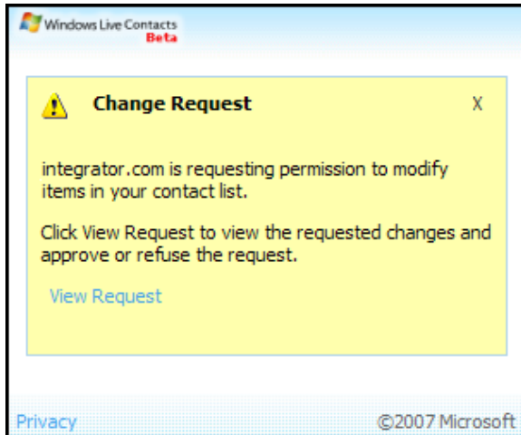
Figure 3: Lowe Anomaly: This Windows Live Contacts gadget received a message that appeared to come from integrator.com , but in reality the request was made by attacker.com .
