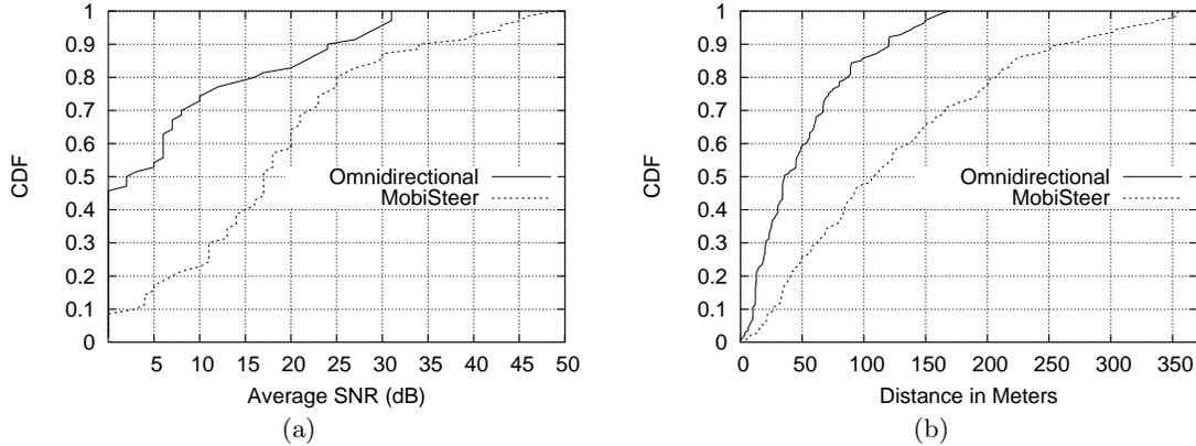
**Figure 13: (a) Average SNR from *In Situ* APs in each 40 meter segment along the route with beam steering and with omni-directional beam. (b) Distance along the route each AP was heard with beam steering and with omni-directional beam.**
