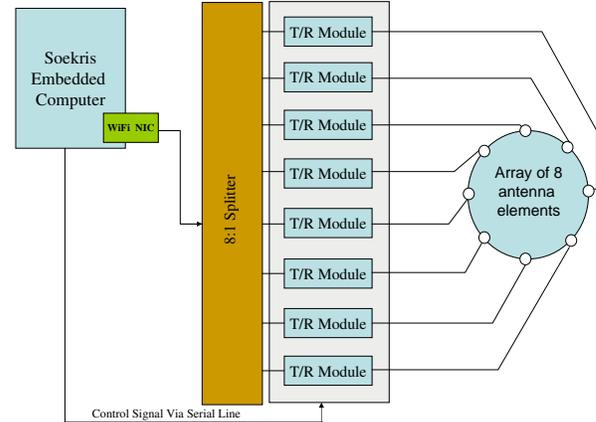
**Figure 2: Block diagram of directional antenna components.**
