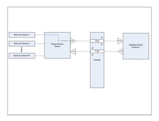
From his description, this is a diagram we created to understand what he was doing. This is the existing system, with a front-end WebSeal webserver, a firewall, the PD authentication server in the middle, providing fine-grained access to various back-end content servers.
