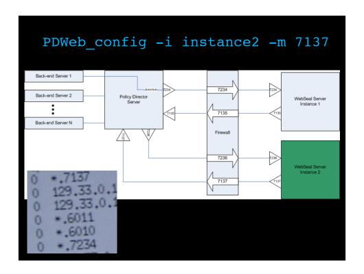
George just saw, then dismissed, the cause of the problem. The machine running instances 1 & 2 is listening on ports 7137 and 7234. But from what George says elsewhere, the incoming ports should be 7234 and 7236. George misunderstood the meaning of the original command-line argument when creating the instance, and his misunderstanding is preventing tech support from helping him.
