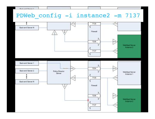
Through analysis of the video and the manuals, we eventually were able to make these pictures. George's view was the top picture, with two ports for each instance. Reality was the bottom picture, with communication on the 7137 port going the other way, and being blocked by the firewall.
