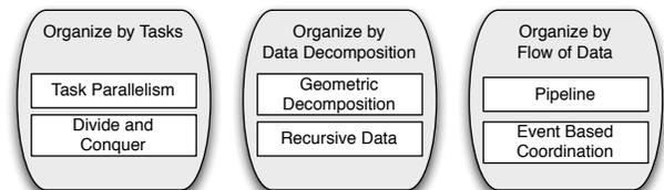
Figure 1 - Algorithmic Parallel Patterns
