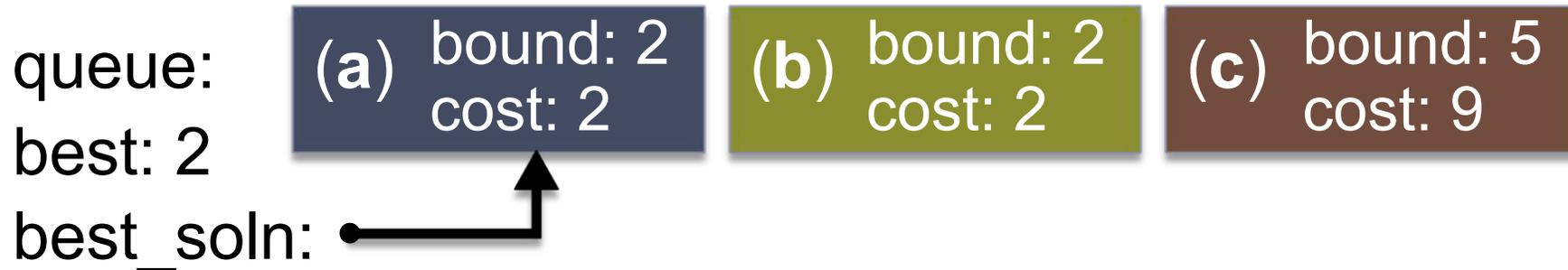
Parallel code can avoid pruning by interleaving iterations. NDSEQ version must prune either **(a)** or **(b)**.
