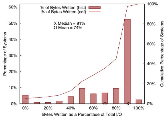
Figure 6: Read/write byte ratio
