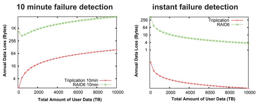
Interaction of parallel repair and detection delay
