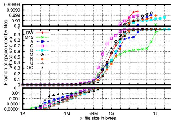
**Figure 1:** The CDF of total capacity used in the files of given size collected from cloud computing clusters (each line represents each cluster). X axis is in log scale of base 4. The Y axis is split into 3 sections. Section from 0 to 100 percentile is linear; section from 90 to 99.999 percentile and 0.001 to 10 percentile is log scale.
