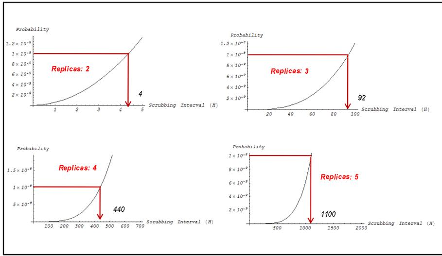
Figure 2. Data Loss Probability vs. Scrubbing Interval
