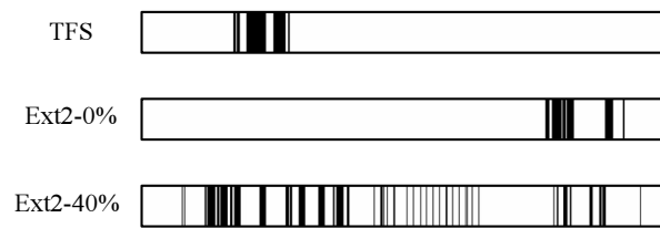
Figure 10: Block allocation pattern for several contribution levels in Ext2 and TFS. Both TFS and Ext2 with 0% contribution show high locality. Ext2 with 40% contribution does not because the contributed files interfere with the block allocation policy.
