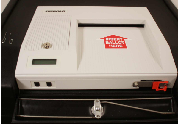
Figure 1: The AccuVote Optical Scan voting terminal (AV-OS). The terminal is shown prior to it being locked to the ballot box, with its front panel visible and showing two control buttons (Yes/No on the lower left corner) and the memory card slot with the card sealed in (lower right corner).
