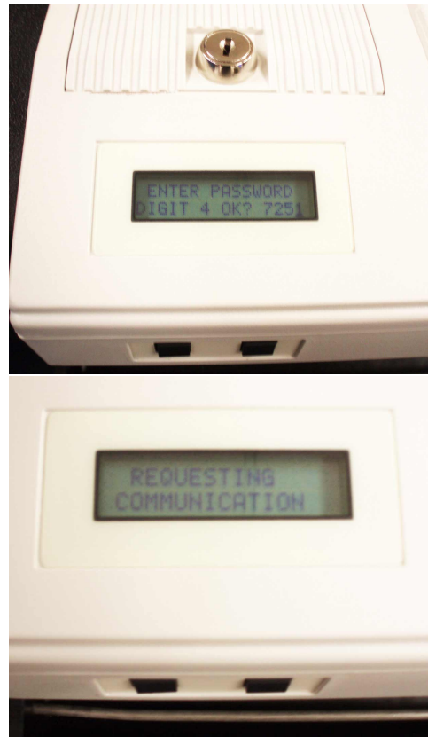
Figure 3: (Left) : The attacker enters the PIN to enter supervisor mode. (Right) : The AV-OS is requesting communication from the GEMS system to overwrite the memory card contents with the forged election setup.
