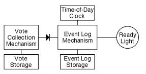
Figure 4: A data diode within a voting machine
