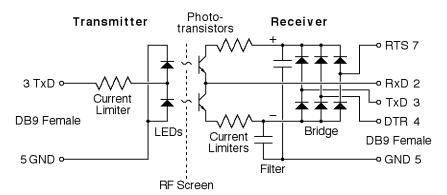
Figure 1: Schematic of the data diode.
