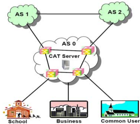
Fig.2. Distributed change detection of DDoS attacks over multiple AS domains.
