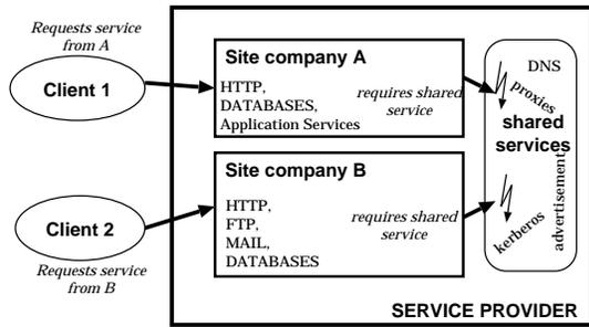
Figure 1: Service-sharing destroys insulation
