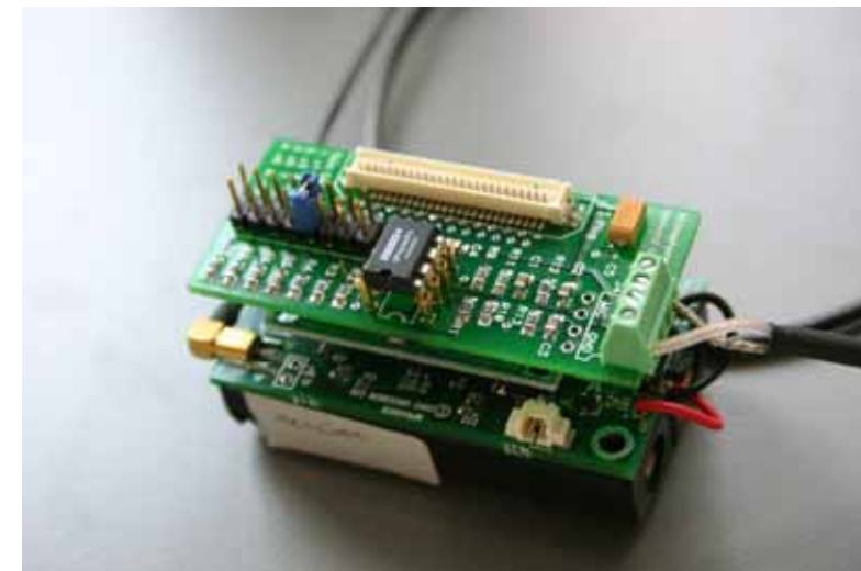
MicaZ with custom infrasonic microphone sensor board
