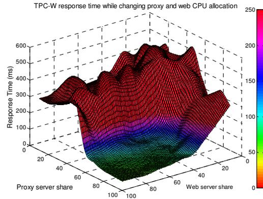
**Figure 7: Proxy and Web tier CPU allocation response times for 40% CPU contention**
