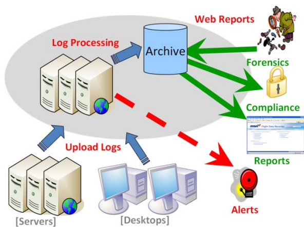
Figure 2: LiveOps System Architecture and data flow.
