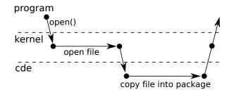
Figure 4: Timeline of control flow between target program, kernel, and cde process during an open syscall.
