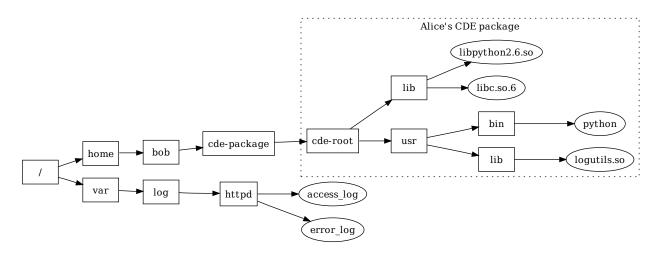
Figure 8: Example filesystem layout on Bob's machine after he receives a CDE package from Alice (boxes are directories, ellipses are files). CDE's seamless execution mode enables Bob to run Alice's packaged script on the log files in /var/log/httpd/ without first moving those files inside of cde-root/.
