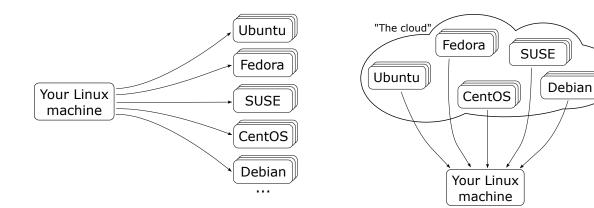
Figure 1: CDE enables users to package up any Linux application and deploy it to all modern Linux distros.
