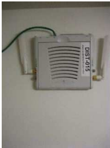
A closed-flap wireless monitor
