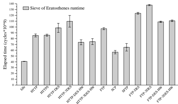
Figure 14: IPsec introduced overhead on the normal performance of a system. Impact on the execution time of CPU intensive job (sieve) on a system that uses IPsec.
