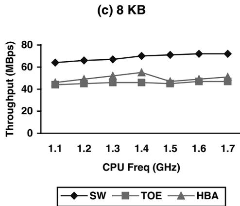
**Figure 3.** This figure shows the sensitivity of the throughput in relation to CPU speeds (denoted in terms of CPU frequency) in each of the three approaches for the block sizes of (a) 0.5 KB, (b) 4 KB, (c) 8 KB, and (d) 64 KB.
