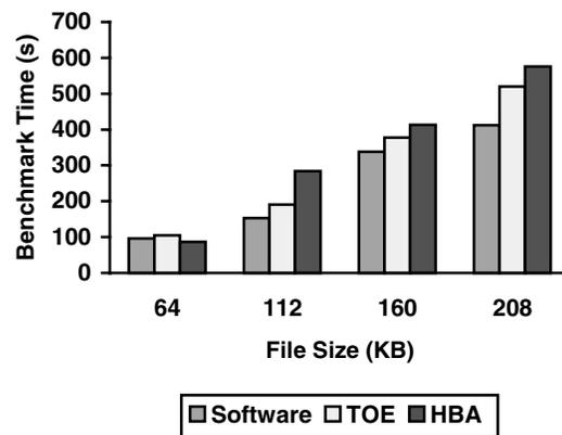
**Figure 6.** This figure shows the time to complete the PostMark benchmark for the three approaches: Software, TOE and HBA when the size for 150 files is varied from 64 KB to 208 KB in increments of 48 KB. The remaining PostMark parameters are the default.
