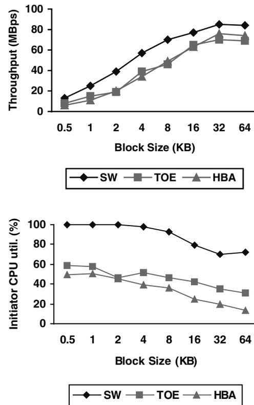
Figure 2. The figure shows the sensitivity of the throughput in each of the three approaches in relation to block size. The resultant initiator workstation CPU utilization is shown on the right.
