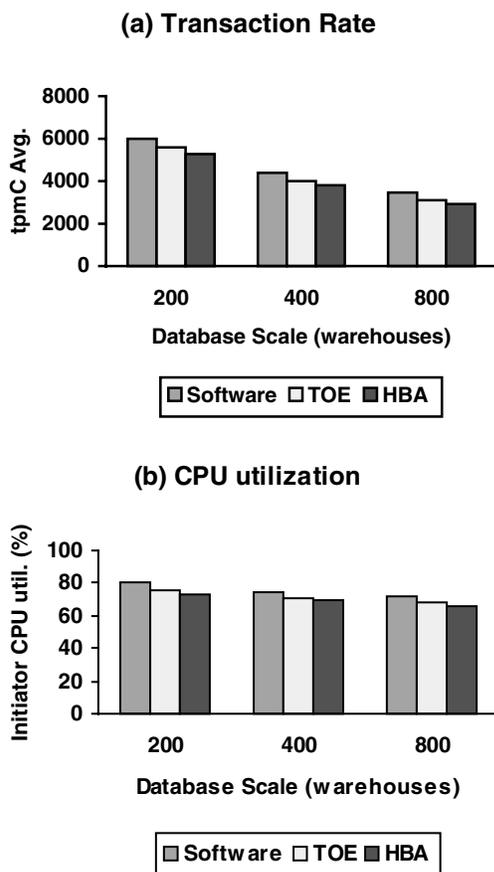
**Figure 5.** (a) This figure shows the average transactions completed per minute for the three approaches: Software, TOE and HBA when running the TPC-C benchmark for a database scale that spans 200 to 800 warehouses. (b) This figure shows the average CPU utilization in the initiator workstation for the experiments described in (a).
