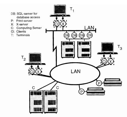
Figure 1. Sample autonomous decentralized system.
