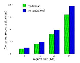
Figure 2: File system response times for a 128 KB file with and without the disk cache performing readahead. The readahead values are measured; the no-readahead values are predicted by the model.
