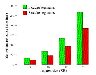
Figure 6: File system response times for 8 64 KB files with 3 and 8 segments. 3-segment values are measured and 8-segment values are predicted by the model.
