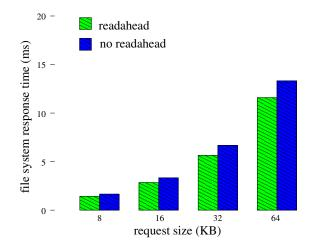
Figure 1: File system response times for a 64 KB file with and without the disk cache performing readahead. The readahead values are measured; the noreadahead values are predicted by the model.
