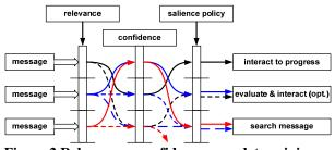
Figure 2 Relevance – confidence map determining the message salience and the associated actions<sup>1</sup>.
