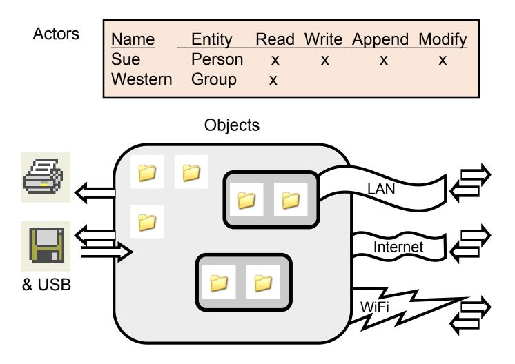
Level 4: Networked PC with files, local printer, local disks, two way
