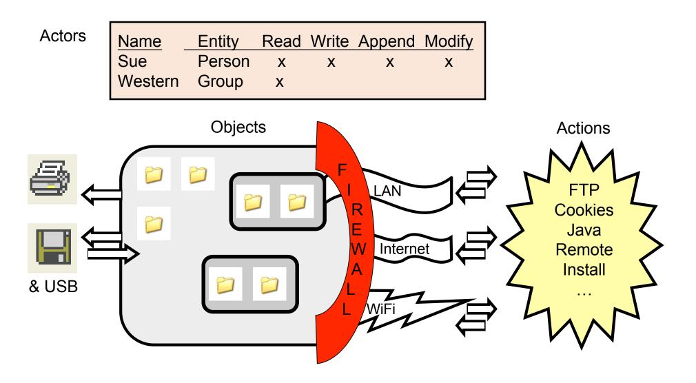
Level 5: Networked PC with files, local printer, local disks, two way
