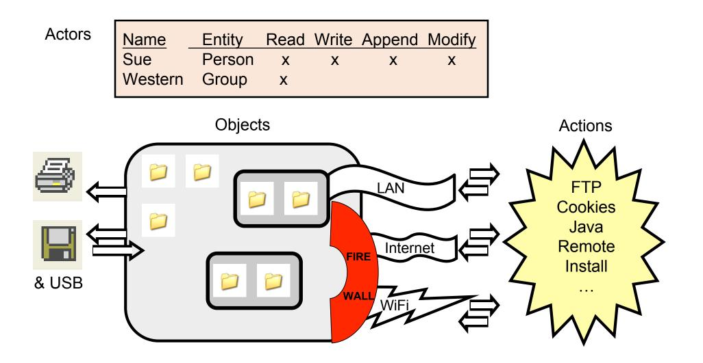
Level 5: Networked PC with files, local printer, local disks, two way
