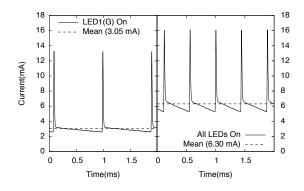
Figure 10: Current over time for two states of Blink recorded with the oscilloscope, showing the mean current and the iCount pulses that Quanto accumulates.
