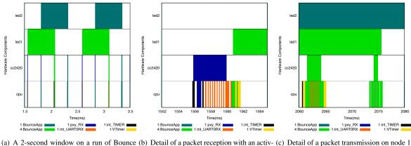
a) A 2-second window on a run of Bounce (b) Detail of a packet reception with an activ- (c) Detail of a packet transmission on node 1 at a node with id 1. ity label from node 4. as part of the activity started at node 4.
