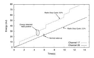
Figure 13: 802.11 b/g interference on the mote 802.15.4 radio. In the top curve the mote was set to the 802.15.4 channel 17, and in the bottom curve, to channel 26. These are, respectively, the closest to and furthest from the 802.11 b channel 6 which was used in the experiment.
