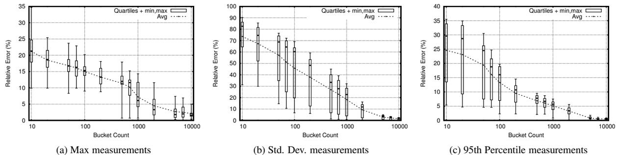
Figure 4: Relative error for DBM-mr algorithm shown for the  $400 \mu\text{s}$  time scale with a varying number of buckets. The box plots show the range of relative errors from the 25th to 75th percentiles, with the median indicated in between. The box whiskers indicate the min and max errors.
