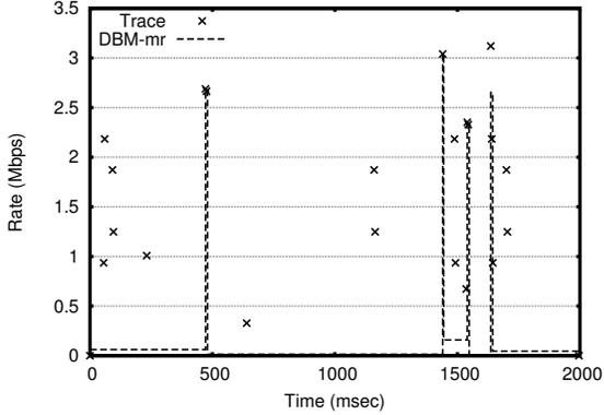
Figure 5: Visualization of events from a 2 second aggregation period overlaid with the output of `DBM-mr` using 9 buckets and a 4 msec measurement time scale.
