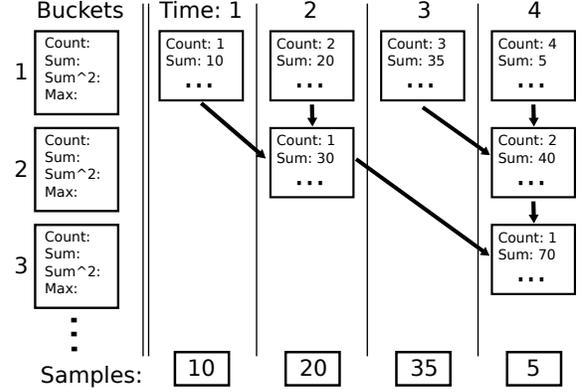
Figure 3: Exponential Bucketing Example. Each of the  $m$  buckets collects statistics at  $2^{i-1}$  times the finest time scale. At the end of each time scale,  $\Delta_i$ , buckets 1 to  $i$  must be updated. Before storing the new sum in a bucket  $j$ , we first add the old sum into bucket  $j + 1$ , if it exists.
