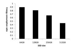
Fig. 1. Energy consumption ratio against the SSD size.
