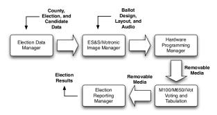
Figure 1: The high level overview of the ES&S Unity voting system with user input to each stage of the election.
