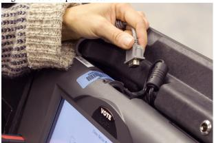
Figure 4: Unhindered access to printer connection allows disabling the iVotronic VVPAT audit log as well as the ability to print unauthorized data to the audit log.
