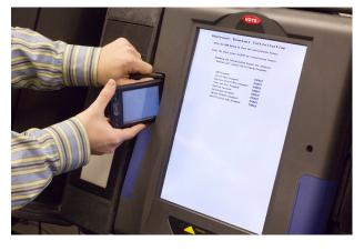
Figure 3: A PEB emulator running on a Palm device simulates an initialization PEB during an open election, resetting all iVotronic passwords.
